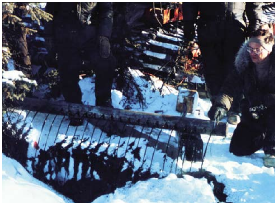
February 26, 1976: experimental crude oil spill in the Caribou-Poker Creeks Research Watershed. Two thousand gallons of hot Prudhoe Bay crude oil were applied through a 30-foot long perforated pipe, shown above.
