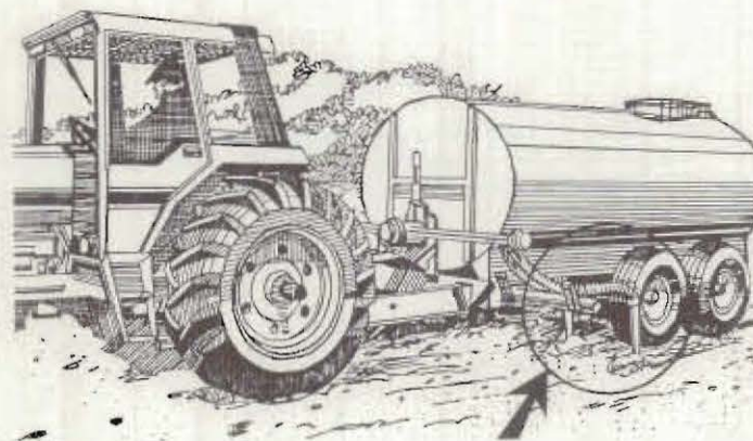
Figure 4. Side-mounted, adjustable, spring-loaded knives inject manure into the soil from the tankwagon.
