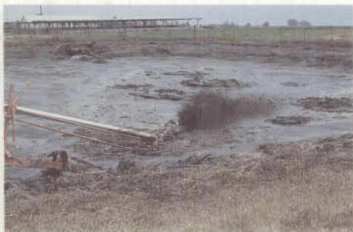
Figure 2. Open-pit pump provides convenience and fastest agitation or pumping from earthen basins.
