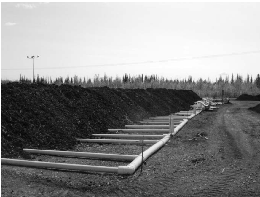
Above: An active pile with PCV piping blowing air into the compost every ten feet. The pipe is unperforated outside of the pile, but perforated in the portion under the pile to ensure good oxygenation.
