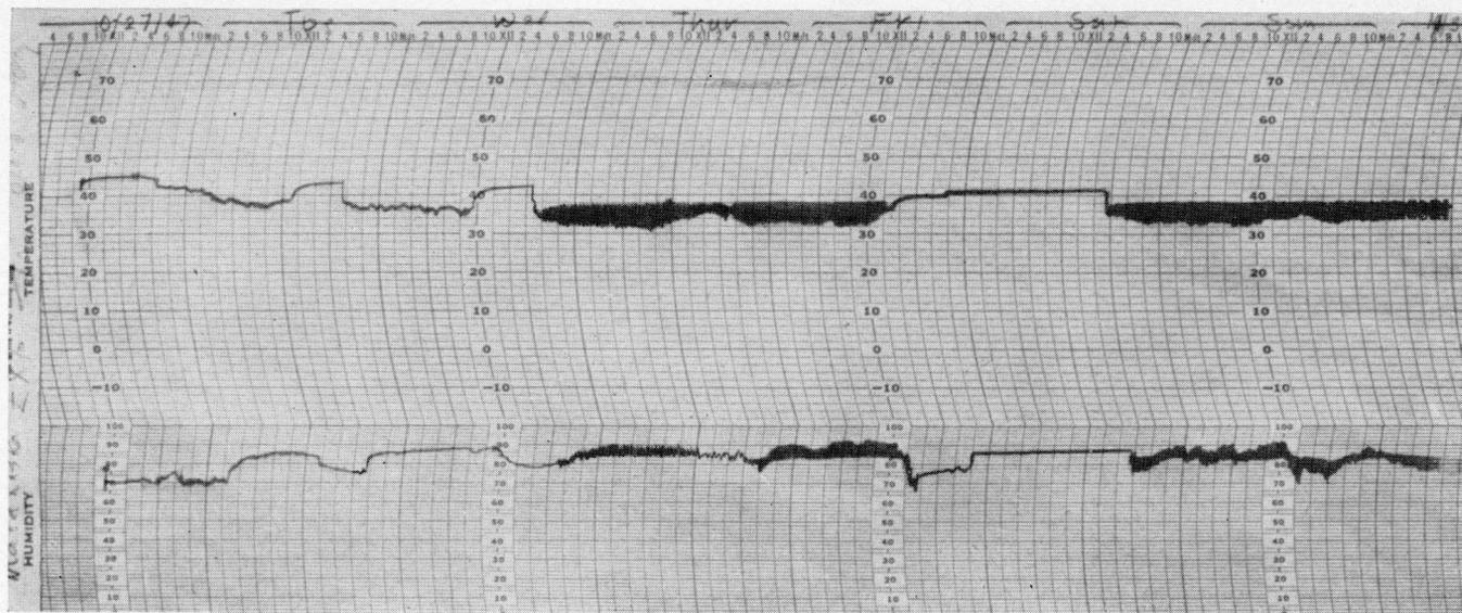
Figure 23.—Chart showing temperature and relative humidity in the Matanuska Experiment Station storage.
