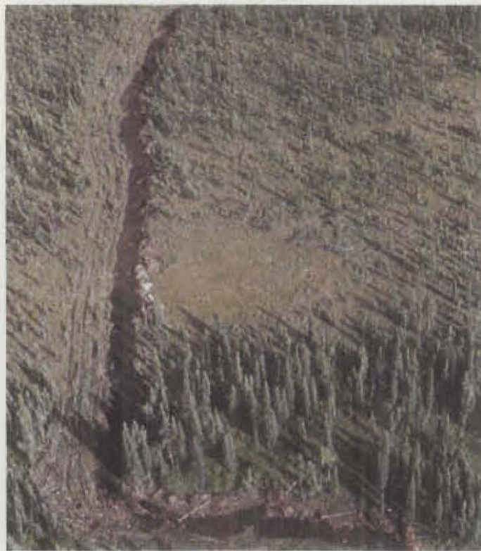
Figure 2. Control lines on the Rosie Creek fire, bulldozer over black spruce permafrost ground. When thawed, such channels fill with water. The insulating vegetative mat was replaced after the fire was controlled.
