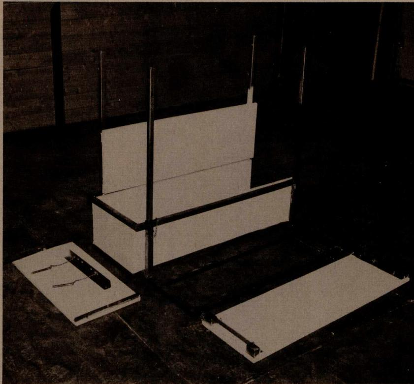
Figure 2 — Collapsible crate for shipping reindeer
